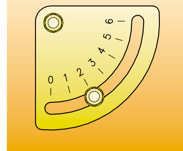
Example of air damper of GI/EMME burners
