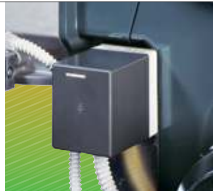
Example of the servomotor for air/gas setting
